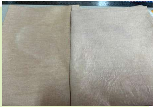
Figure 12. Uneven distribution of colour tones on hand-dyed fabric after drying © Chuen Mun Wai
