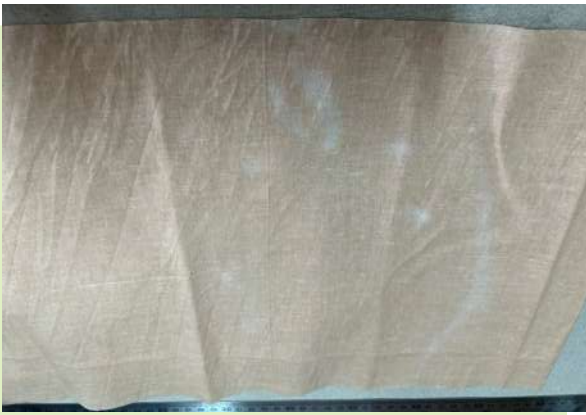
Figure 11. Excessive humidity can result in the formation of white spots on the cloth © Chuen Mun Wai
