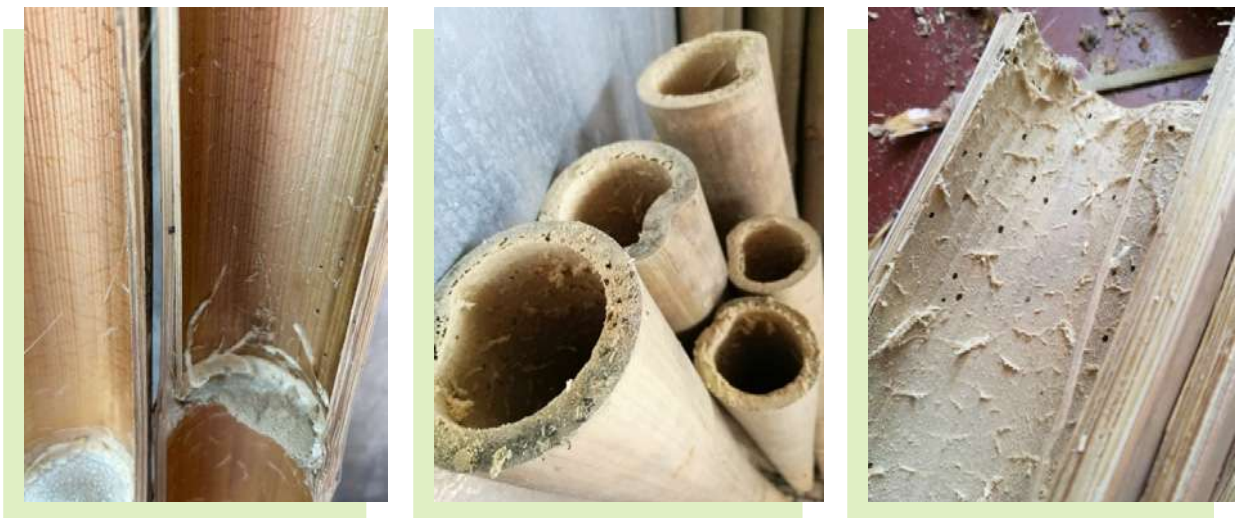
Figure 9. Defective bamboo logs with small holes, a result of infestation by ants, spiders and scorpions © Chuen Mun Wai
