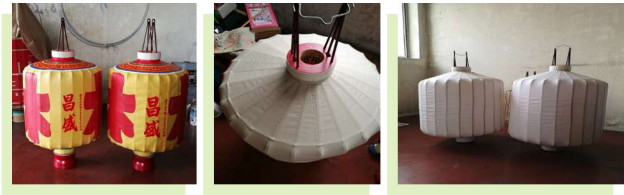
Figure 13. Imperfections on lantern fabric covers: Wrinkles in the cloth due to excessively rapid drying or changes in the glue that attaches the cloth to the frame or to the adhesive layer applied on the cloth surface. These occur in situations of high temperatures and high rainfall and humidity © Chuen Mun Wai
