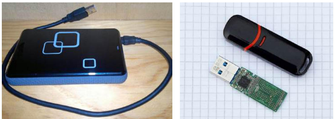
Images, left: A USD-attached solid state drive. Right: The components inside a flash thumb drive Source: Pixabay (public domain)
