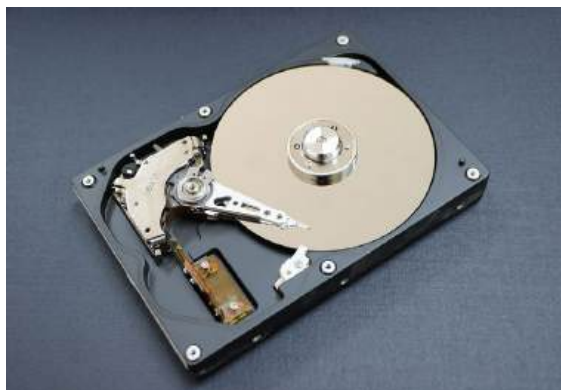
Image: The interior of a hard drive, showing the actuator arm and the disk that spins Source: Pixabay (public domain)
