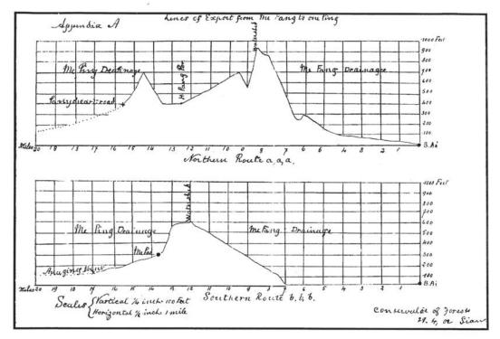
Figure 2 A route plan for teak timber "exports" from the Fang River to the Ping River (Source: NA r5 M 16.1/23 Mae Ing Forests in relation to France, 28 Jan. 1902)
