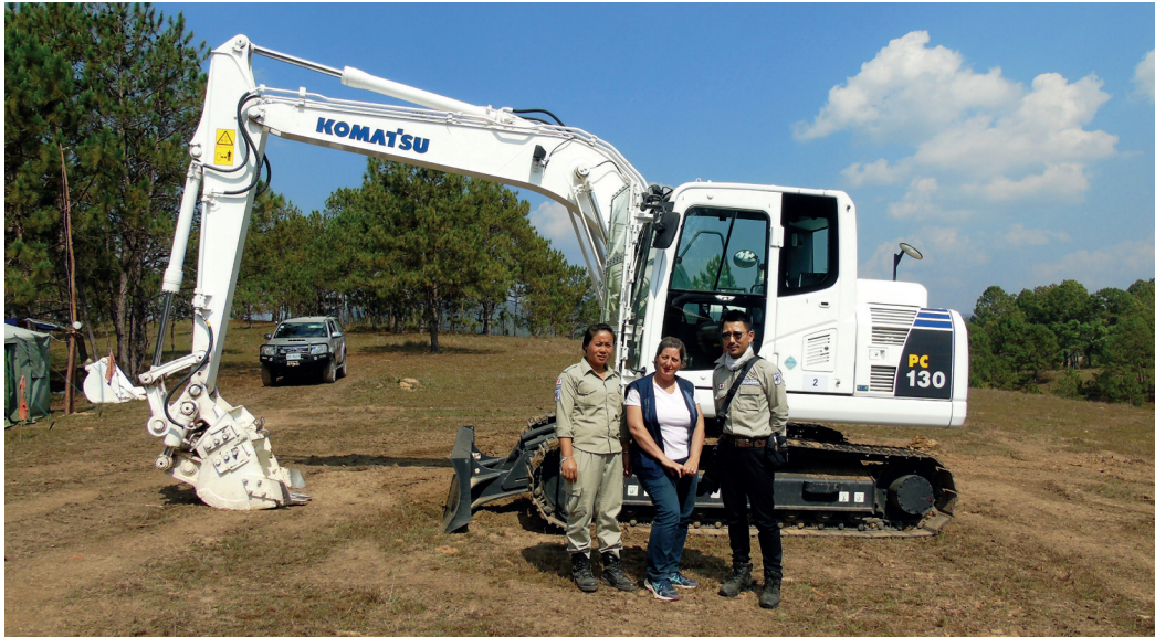
Figure 6. JMAS (Japan Mine Action Service) has conducted demining operations in Laos since 2005. The PC 130 in the picture was specially modified for clearance work in Xieng Khouang. L-R: Khambay Saiyavongsar (UXO-Lao Senior explosive ordnance disposal technician), Lia Genovese, Hideki Kamei (JMAS Technical advisor). (Photo: Lia Genovese).
