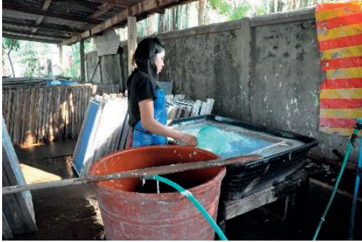
Figures 17a, b. The paper sheet formation method with fixed mold made with a plastic screen attached to a wooden frame observed in Say Namkhan Company in Luang Prabang. It is the floating method characterized by the pouring of paper pulp directly on the sieve in carefully measured scopes (similarly to a technique widely used in the Himalayas). © Agnieszka Helman-Ważny.
