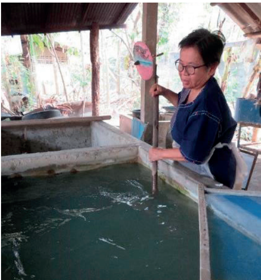
Figures 18a, b. The paper sheet formation method with a fixed mold made with a plastic screen attached to the wooden frame in Sa Paper & Umbrella Handicraft Factory, Chiang Mai. Considering the technology, it is the dipping method characterized by the paper pulp being derived from all the volume of the water tank (opposite to the above technique observed in Laos when the pulp is poured directly onto the sieve in carefully measured scopes). © Agnieszka Helman-Ważny.
