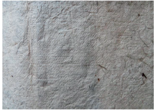
Figure 20. Texture of paper showing the print of a papermaking sieve in the manuscripts from the Buddhist Archives in Luang Prabang archived as Nan Savaeng ms 2 . © Agnieszka Helman-Ważny.
