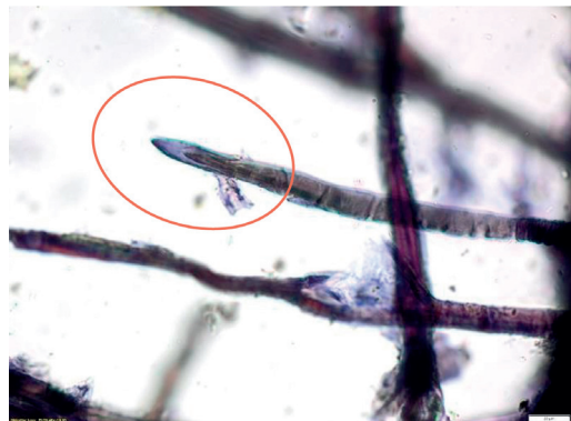
Figure 13b. The natural blunt end of a Paper mulberry fiber after treatment with Herzberg stain observed under the microscope at 400× magnification in the manuscript archived as BAD 13-2-021 from the Buddhist Archives in Luang Prabang. © Agnieszka Helman-Ważny.
