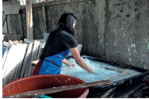
Figures 17a, b. The paper sheet formation method with fixed mold made with a plastic screen attached to a wooden frame observed in Say Namkhan Company in Luang Prabang. It is the floating method characterized by the pouring of paper pulp directly on the sieve in carefully measured scopes (similarly to a technique widely used in the Himalayas). © Agnieszka Helman-Ważny.
