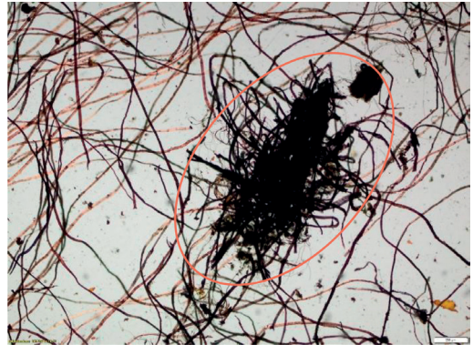
Figure 14. The 'knot' of other fibers stained violet among Paper mulberry-based pulp observed at 40× magnification in the manuscript archived as CMRU ms 1 from Chiang Mai Rajabhat University Library. © Agnieszka Helman-Ważny.
