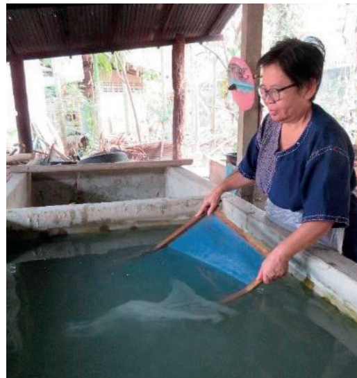
Figures 18a, b. The paper sheet formation method with a fixed mold made with a plastic screen attached to the wooden frame in Sa Paper & Umbrella Handicraft Factory, Chiang Mai. Considering the technology, it is the dipping method characterized by the paper pulp being derived from all the volume of the water tank (opposite to the above technique observed in Laos when the pulp is poured directly onto the sieve in carefully measured scopes). © Agnieszka Helman-Ważny.
