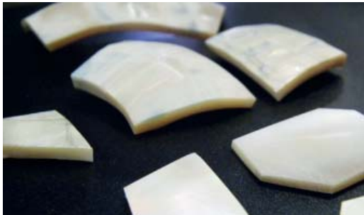
Figs. 14-16 (above). The shells were first cleaned and smoothed using grinding machines to remove the brownish-green, rough outer surface until the inner glossy white and pink part was reached.
