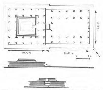
Figure 7. Plan and elevation and east profiles of the Candi Bukit Batu Pahat (SMK 1(8w), South Kedah, Malaysia.
