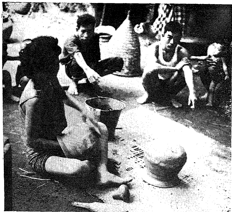
Plate VII Ban Nong pottery manufacture; a forming bottom of pot; b in foreground a girl playing a pottery drum with a moist cloth for drumhead; front foreground, broken jars used to support large jars while drying; background, pottery in different stages of manufacture, under house in back are dry jars ready for firing.
