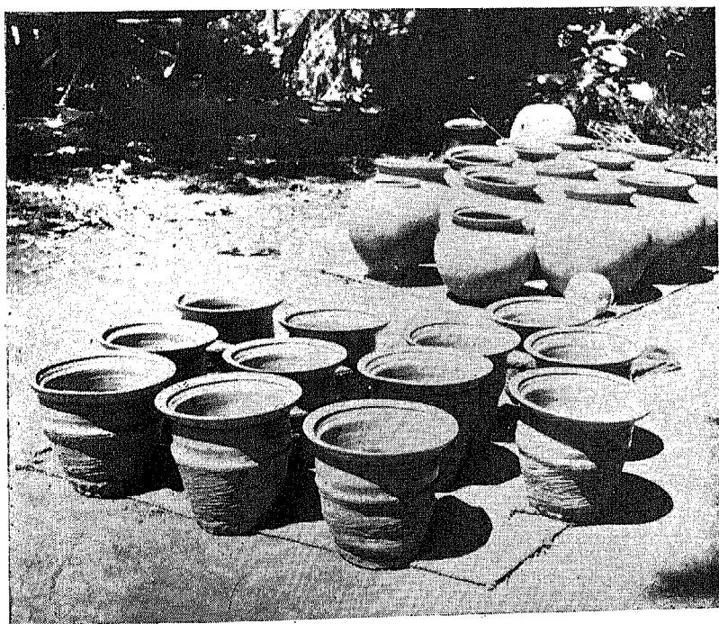
Plate V Ban Nong pottery manufacture: a forming the rim; b pots drying in the sun, in the foreground with rim completed but body not yet begun, in background completed jars.
