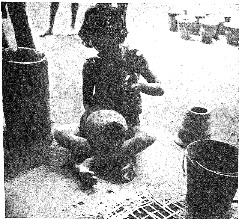
Plate VI Ban Nong pottery manufacture: a-b closing the bottom of the hollow cylinder and expanding the body.
