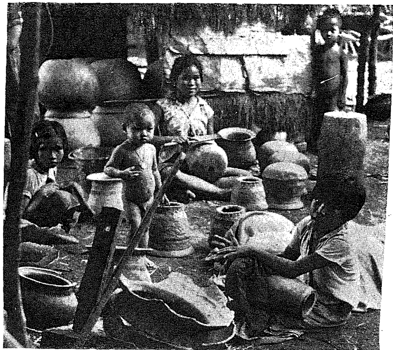
Plate VII Ban Nong pottery manufacture; a forming bottom of pot; b in foreground a girl playing a pottery drum with a moist cloth for drumhead; front foreground, broken jars used to support large jars while drying; background, pottery in different stages of manufacture, under house in back are dry jars ready for firing.
