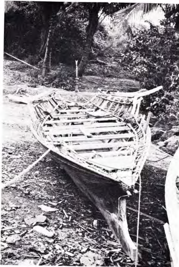
View from the bow of a Moken kabang. Note the step cut in the bow, the framing for the decking with a low bulwark above it, the framework for the sides of the deckhouse including the cradles for masts, oars, bamboos, etc.
