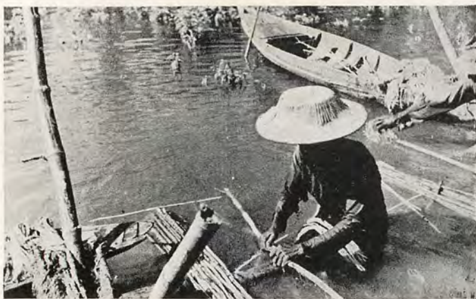
Fig. 10. Holding a retted jute stock near the middle in both hands, the brittle core is broken. Taking one half in one hand, the core is pushed out with the thumb of the other and vice versa, so that the fibre alone is left. This is laid across the lap until a handful is ready for rinsing.
