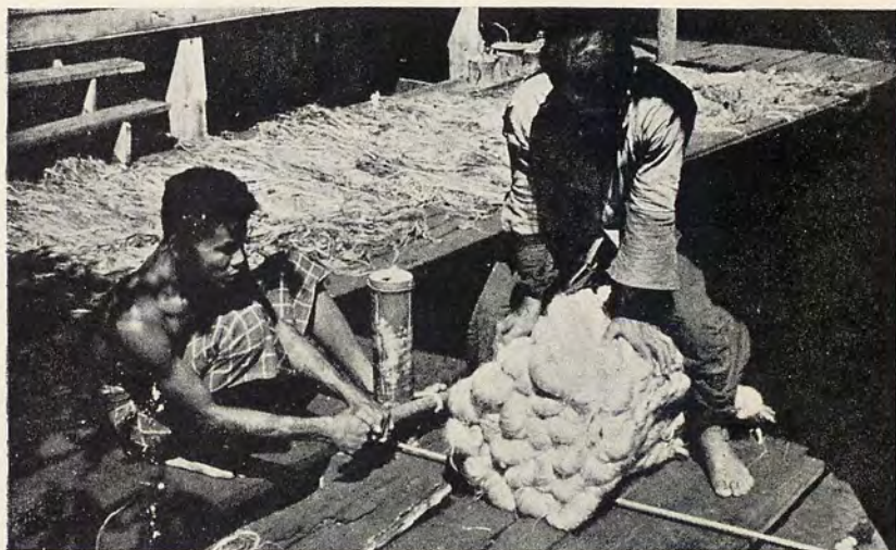
Fig. 13. The method of tying jute fibre into small bundles before transportation. The rope which goes round the bundle is pulled by one man with a simple device, while the other takes a string made from unretted jute bark and fastens it round the bundle.
