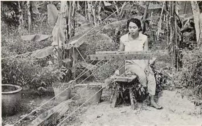
Fig. 6. Twisting the cords, shown in Fig. 5, into ropes.
