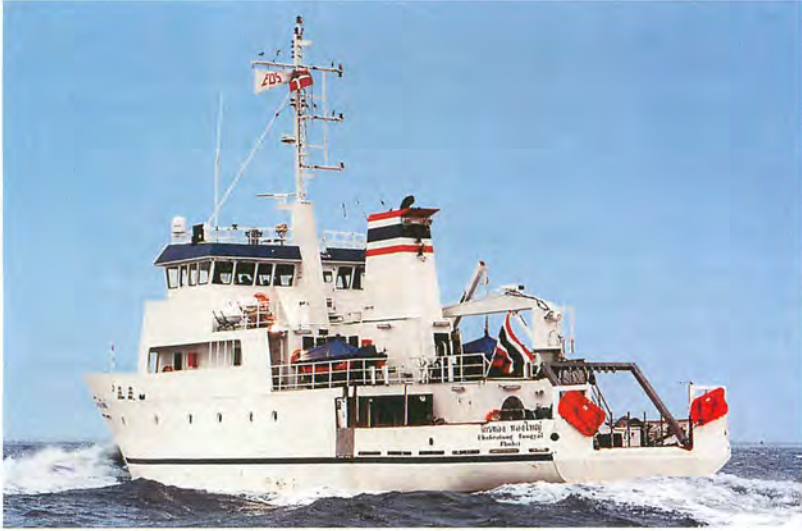
Figure 15. The DANIDA-sponsored Chakratong Tongyai was named after Minister of Agriculture and Cooperatives, M. C. R. Chakratong Tongyai, the first Chairman of the Commission Board of PMBC. The tonnage (GT) is 464, length 38.4 m and width 9 m. The ship is owned by the Thai Department of Fisheries and allocated to operate in waters attached to the PMBS.
